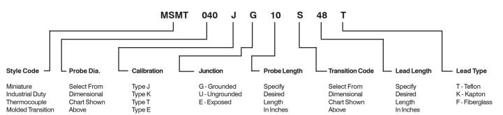
The product code example shown above defines a Style "MSMT" thermocouple with a probe diameter of .040 inches in a type "J" calibration with grounded junction and 10 inch probe length. A stock transition diameter was selected. A 48 inch lead length was specified in the standard Teflon insulated construction.
