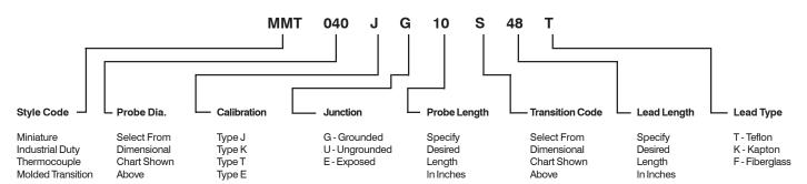
The product code example shown above defines a Style "MIDM" thermocouple with a probe diameter of .040 inches in a type "J" calibration with grounded junction and 10 inch probe length. A stock transition diameter was selected. A 48 inch lead length was specified in the standard Teflon insulated construction.
