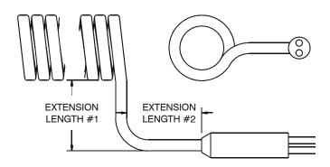
Type "T90" Tangential Extension Exit With 90° Bend
